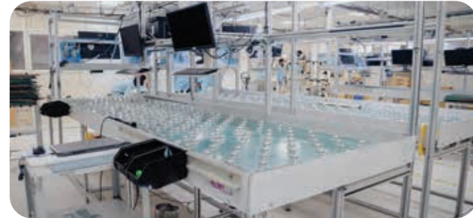
Ball Conveyor Line
