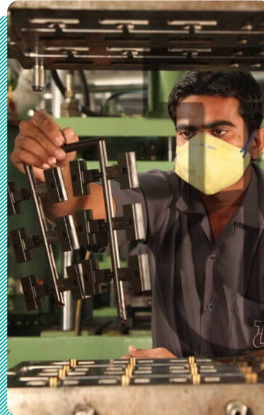
Wax Injection & Pattern Assembly
