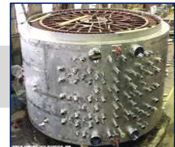
Calandria A tank which is the core of the reactor
