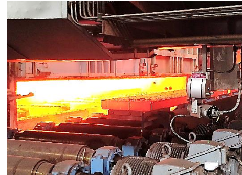
Slab Extraction in HSM at JVML-Vijayanagar
