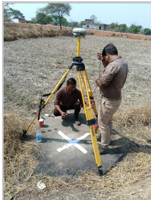
Figure 1: Establishing the survey base station for drone magnetic survey.
