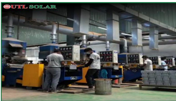
Grid casting set-up for lead acid batteries
