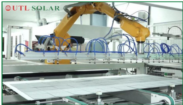
Robotic lay-up for solar panels
