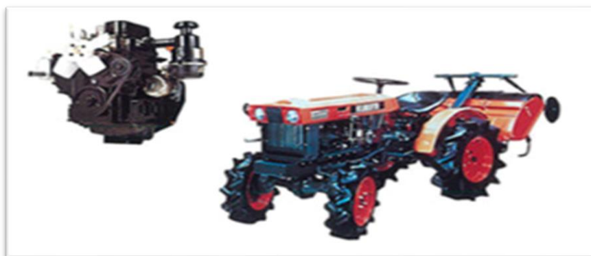
Fig 15 – Ultra-compact 4-wheel drive tractor Bulltra B6000 (right) and its vertical 2-cylinder diesel engine (left)
